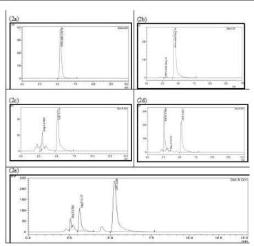
Fig 2 HPLC chromatogram of standard CNT and degradation products of CNT at different degradation conditions
